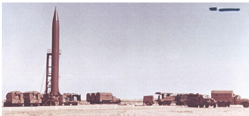
Fig. 1.46. Photo of the missile type R-5M (SS-3 Shyster in NATO classification) with a crossed-out "Top Secret" label during pre-launch preparation on Kapustin Yar range.
