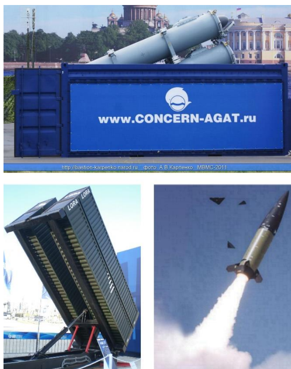
Fig. 1.55. Container-based launching units of missile complexes Club-K (above) and LORA (below).
