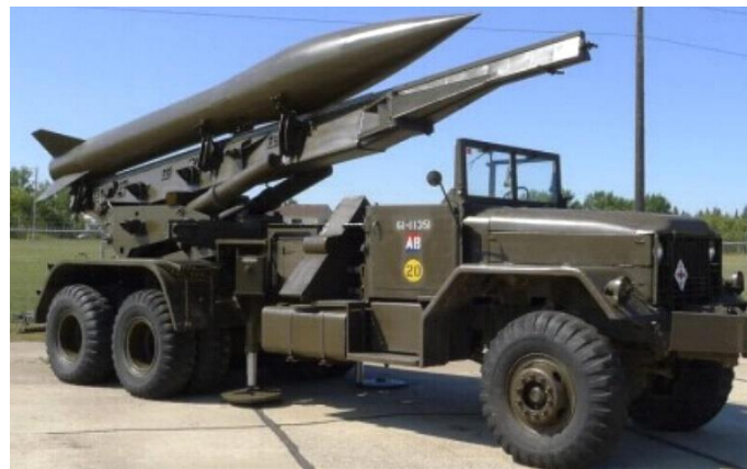
Fig. 1.42. Missile launcher with Honest John (MGR-1) with an over-caliber warhead for nuclear warhead option.
